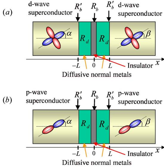
FIG. 1. (Color online) Schematic illustration of the models of (a)  $D/DN//I/DN/D$  and (b)  $P/DN//I/DN/P$  junctions.
