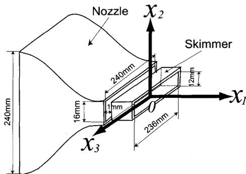
Fig. 1 The skematic of the experimental apparatus near the nozzle exit and the coordinate system
