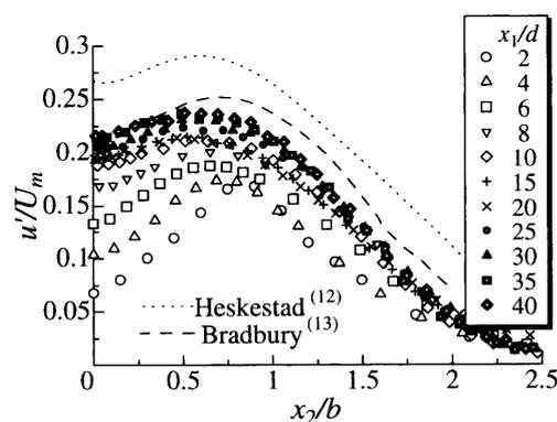
Fig. 3 The cross-streamwise profiles of  $u'$
