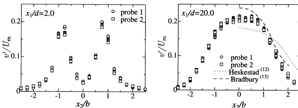
Fig. 9 The profiles of the r.m.s. values of the cross-streamwise velocity  $v'$  for the two-point measurements
