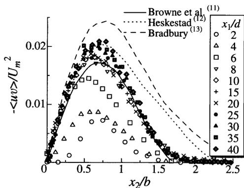
Fig. 5 The cross-streamwise profiles of  $-\langle uv \rangle$
