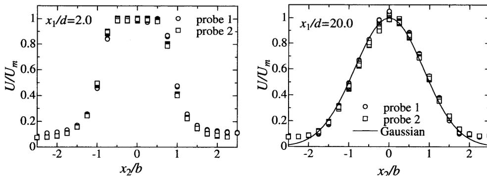
Fig. 7 The profiles of the streamwise mean velocity  $U$  for the two-point measurements
