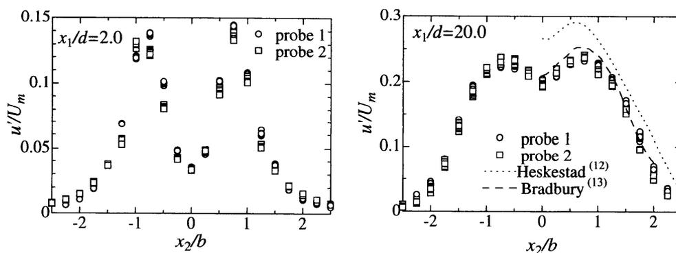
Fig. 8 The profiles of the r.m.s. values of the streamwise velocity  $u'$  for the two-point measurements
