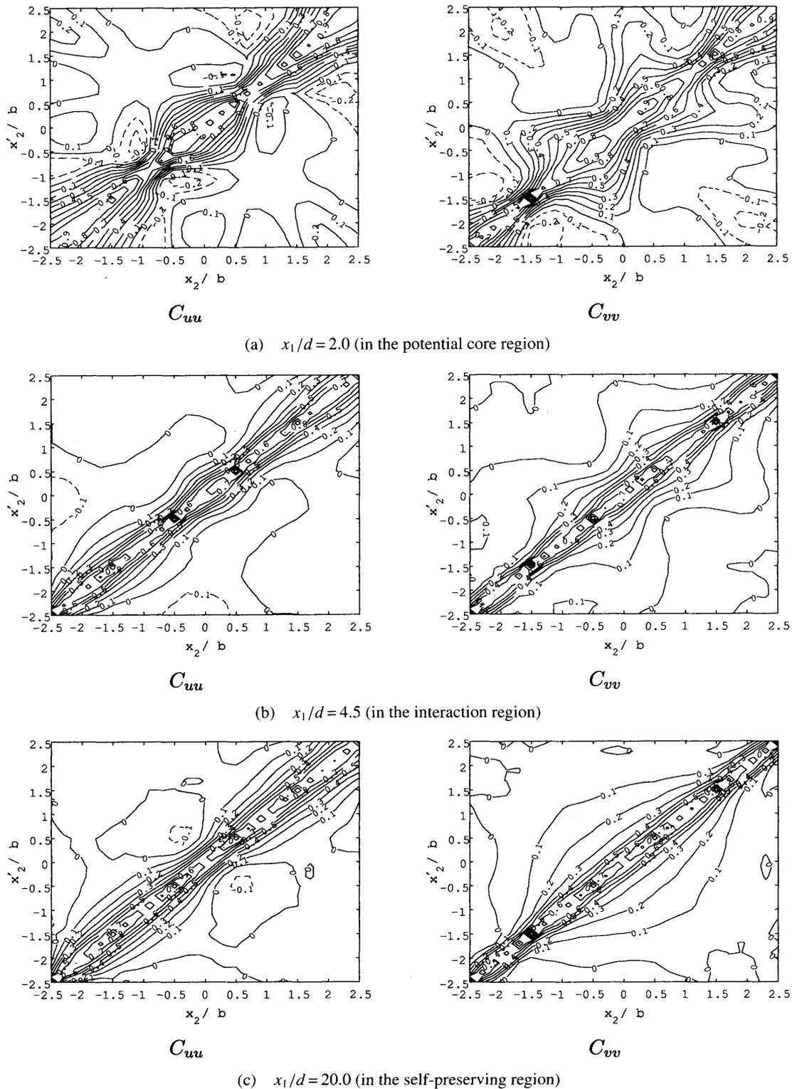
Fig. 10 The downstream variations of the spatial correlation coefficient  $C_{uu}$ ,  $C_{vv}$
