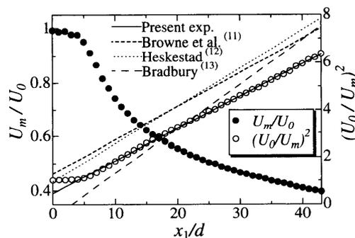
Fig. 2 Axial variation of centerline mean streamwise velocity  $U_m$
