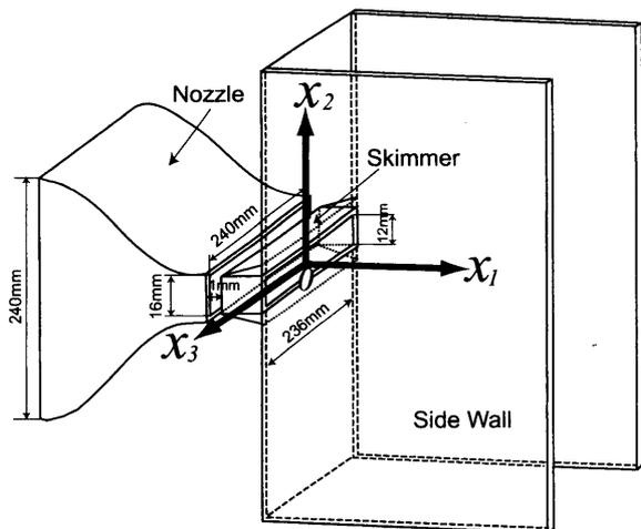
Fig. 1 Schematic of the experimental apparatus near the nozzle exit and the coordinate system
