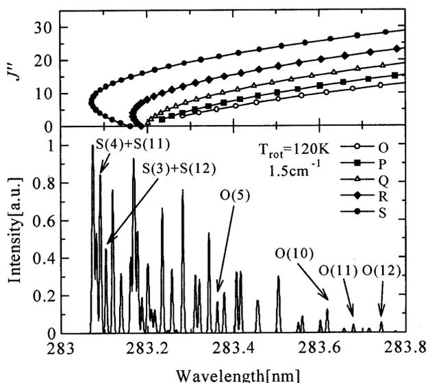
Fig. 7 Simulated REMPI spectrum at  $T_{rot}=120$  K (laser linewidth:  $1.5\text{ cm}^{-1}$ )
