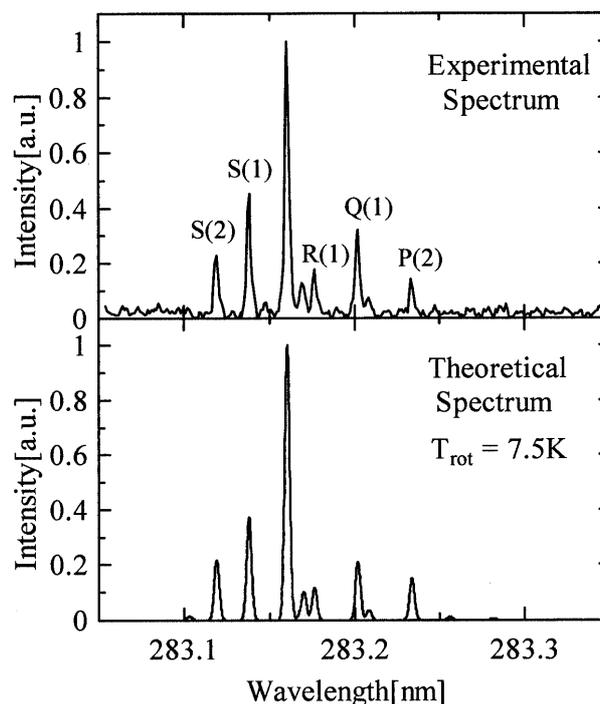
Fig. 4 Experimental spectrum at  $x/D=83$  compared with the theoretical one at  $T_{rot}=7.5 \text{ K}$
