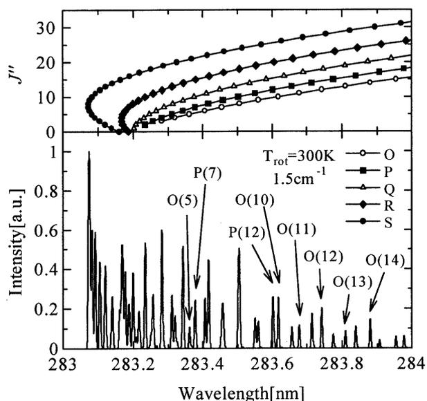
Fig. 8 Simulated REMPI spectrum at  $T_{rot}=300$  K (laser linewidth:  $1.5\text{ cm}^{-1}$ )
