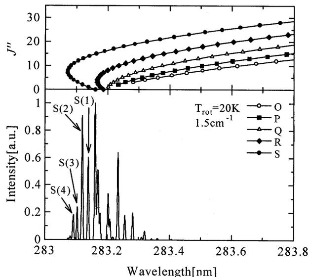
Fig. 6 Simulated REMPI spectrum at  $T_{rot} = 20 \text{ K}$  (laser linewidth:  $1.5 \text{ cm}^{-1}$ )
