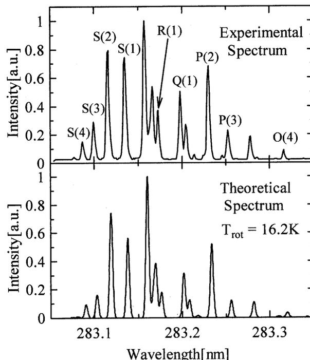
Fig. 3 Experimental spectrum at  $x/D=17$  compared with the theoretical one at  $T_{rot}=16.2 \text{ K}$
