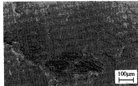
(b) Enlargement of A (fracture surface near an artificial defect)
