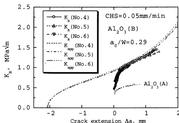
Fig. 20  $R$ -curve behavior for porous  $\text{Al}_2\text{O}_3$  (B)
