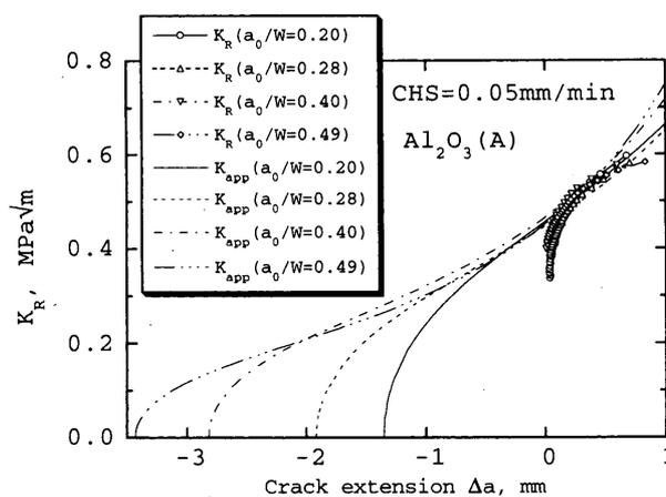
Fig. 17 R-curve behavior for porous  $Al_2O_3(A)$
