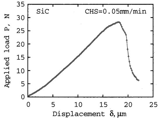
Fig. 9 Applied load vs. displacement curve for SiC
