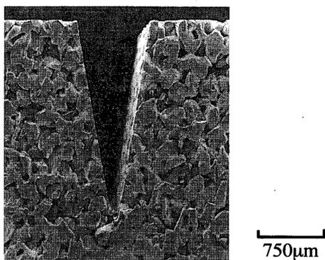
Fig. 3 V-notch in the SEVNB specimen of porous SiC
