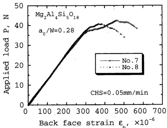
Fig. 22 Applied load vs. back-face strain curve of  $\text{Mg}_2\text{Al}_4\text{Si}_5\text{O}_{18}$
