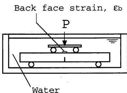
Fig. 4 Schema of the SEVNB method in water
