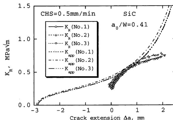
Fig. 12  $R$ -curve behavior for porous SiC
