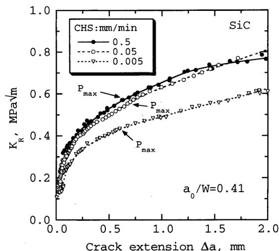
Fig. 13  $R$ -curve behavior for porous SiC under several crosshead speeds
