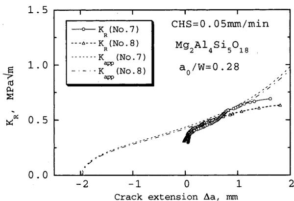
Fig. 23  $R$ -curve behavior for porous  $\text{Mg}_2\text{Al}_4\text{Si}_5\text{O}_{18}$
