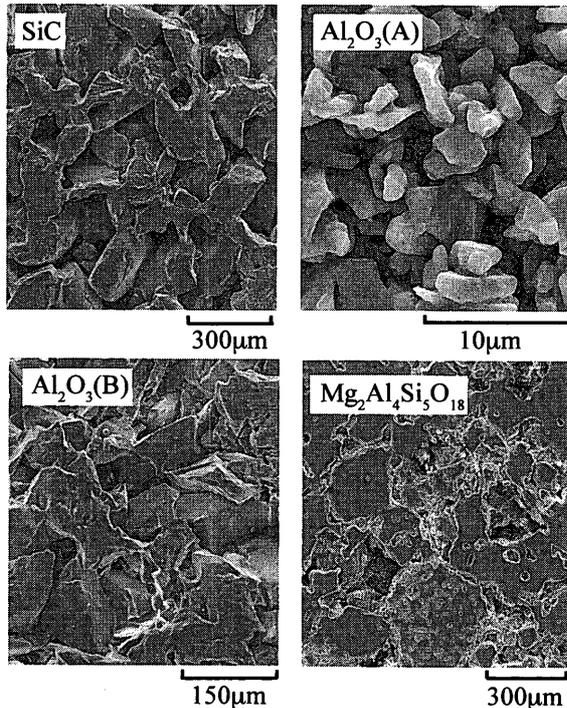
Fig. 1 Microstructures of porous ceramics
