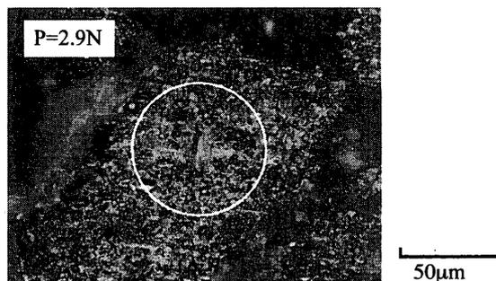
Fig. 5 Micrograph of Vickers indent in porous SiC
