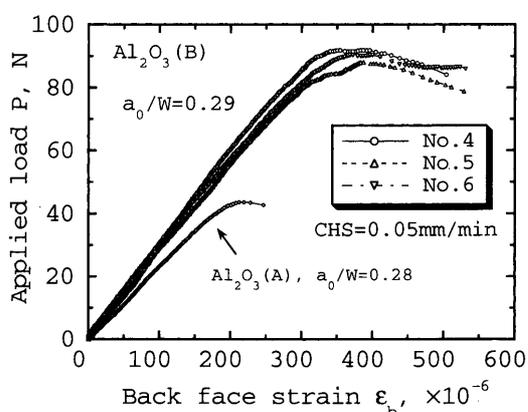
Fig. 19 Applied load vs. back-face strain curve of  $\text{Al}_2\text{O}_3$  (B)
