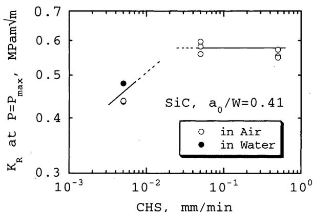
Fig. 15 Relationship between  $K_R$  and crosshead speed
