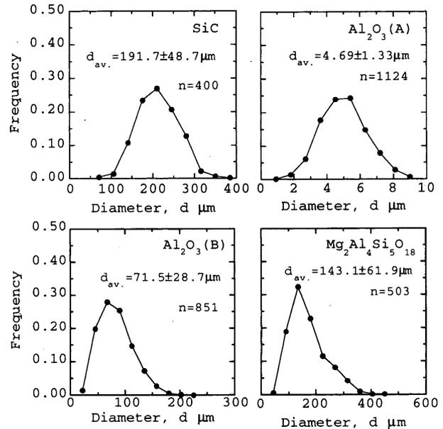
Fig. 2 Distribution in grain diameter of porous ceramics
