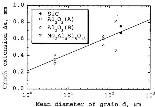
Fig. 25 Relationship between crack extension  $\Delta a$  and grain diameter  $d$  for porous ceramics
