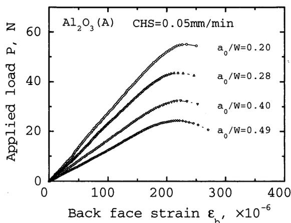
Fig. 16 Applied load vs. back-face strain curve of  $Al_2O_3(A)$
