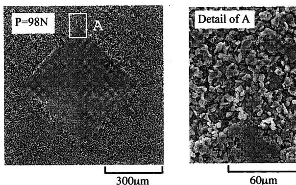
Fig. 6 Micrograph of Vickers indent in porous  $\text{Al}_2\text{O}_3$  (A)
