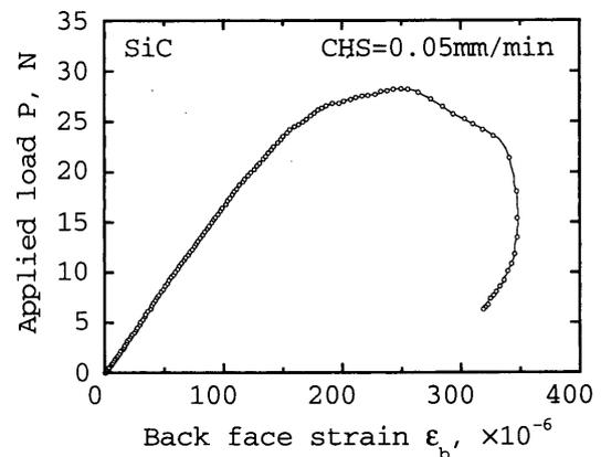
Fig. 10 Applied load vs. back-face strain curve for SiC
