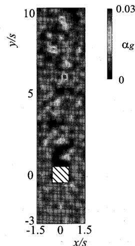
Fig. 7 Distribution of air volumetric fraction at  $t^* = 84$  in case of  $\alpha_{g0} = 0.01$
