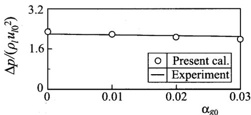
Fig. 11 Pressure difference between front and rear stagnation points of cylinder
