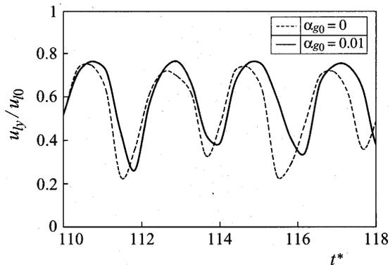
Fig. 9 Time variation of water velocity at point P
