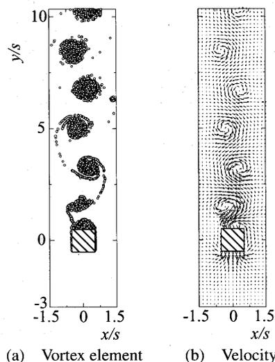
Fig. 4 Water single-phase flow field at  $t^* = 100$
