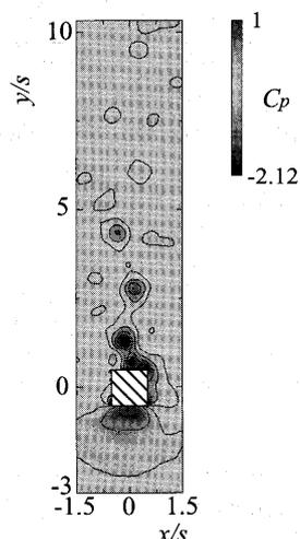
Fig. 8 Pressure distribution at  $t^* = 84$  in case of  $\alpha_{g0} = 0.01$
