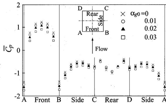
Fig. 12 Pressure distribution on cylinder
