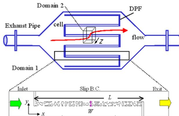
Figure 2 Schematics of DPF system and calculation domain with coordinate.
