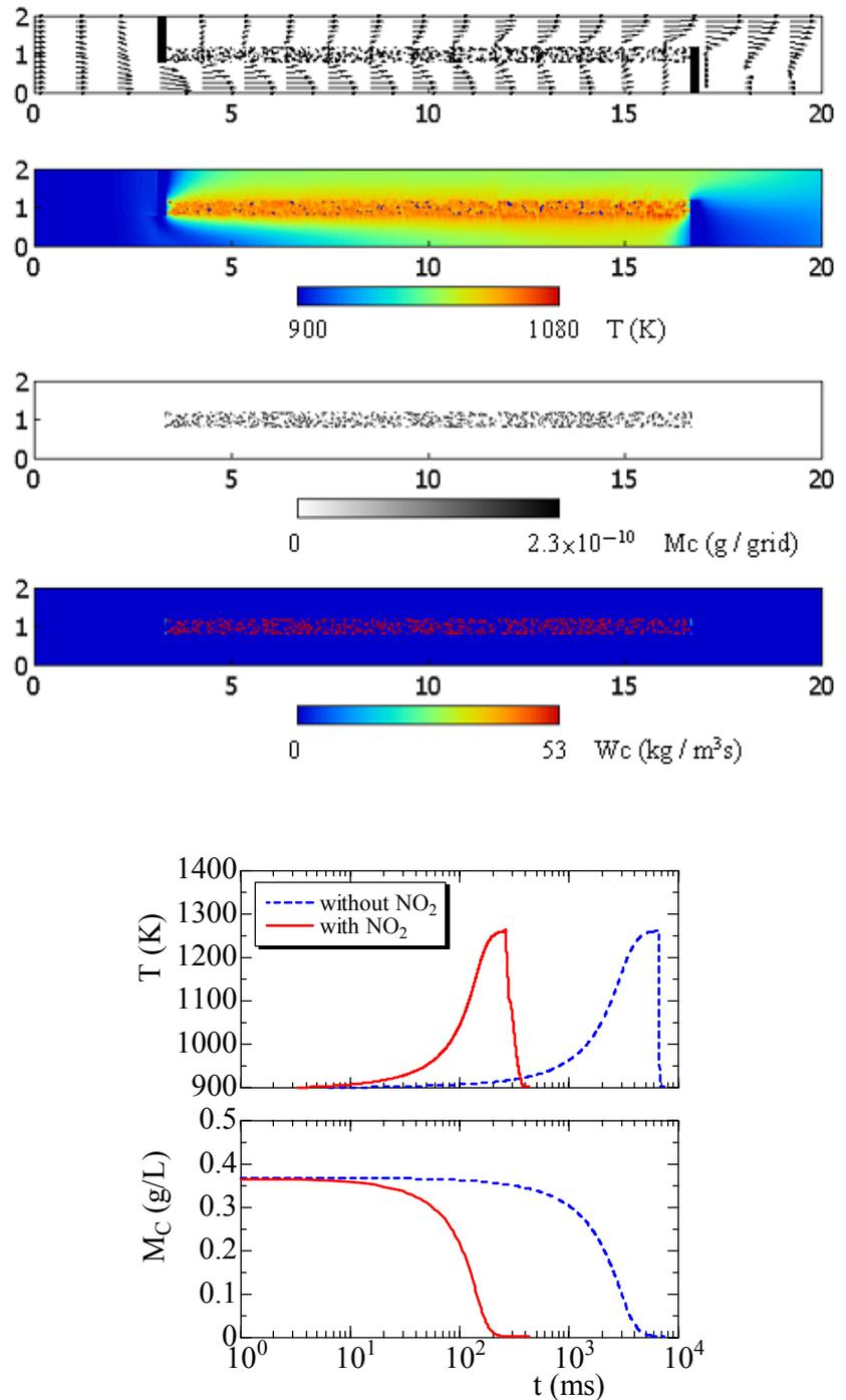
Figure 9 Maximum temperature and mass of remained soot in DPF for  $e = 0.6$ ,  $L = 13\text{mm}$ ,  $d = 33 \mu\text{m}$ ,  $U_0 = 10 \text{ cm/s}$  to observe effect of  $\text{NO}_2$  on soot oxidation.
