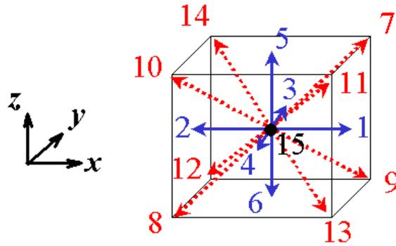
Figure 1 D3Q15 model for 3D simulation.
