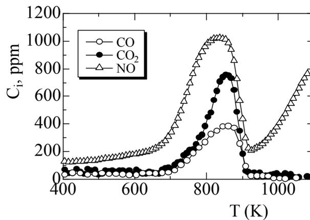
Figure 3 Concentration of products at temperature programmed reactions (TPR) in 1000 ppm  $\text{NO}_2$  + 7%  $\text{H}_2\text{O}$  + 10%  $\text{O}_2$  in  $\text{N}_2$ .
