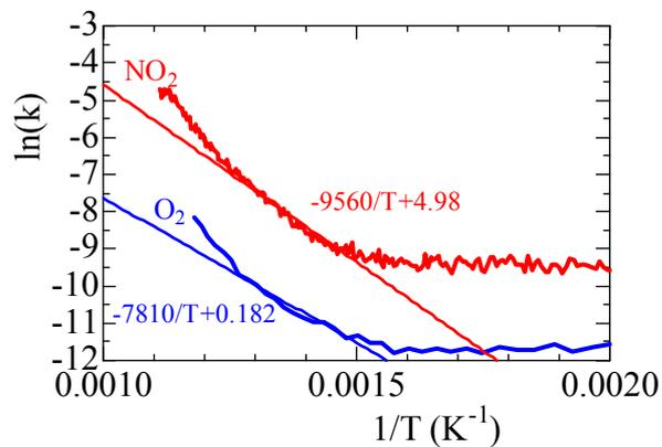
Figure 4 Arrhenius plotting at temperature programmed reactions (TPR) with and without  $\text{NO}_2$ .
