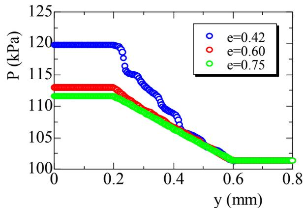
Figure 7 Pressure distributions across filter wall for  $e = 0.42, 0.6, \text{ and } 0.75$ ;
