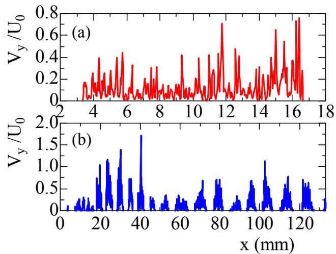
Figure 6 Profiles of velocity passing through porous wall for  $e = 0.6$ ,  $d = 33\ \mu\text{m}$ ; (a)  $L = 13\ \text{mm}$ ,  $U_0 = 10\ \text{cm/s}$ , (b)  $L = 133\ \text{mm}$ ,  $U_0 = 100\ \text{cm/s}$ .
