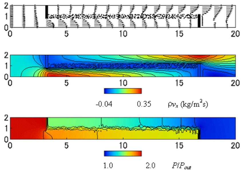
Figure 5 Velocity field in DPF for  $e = 0.6$ ,  $L = 13\text{mm}$ ,  $d = 33\ \mu\text{m}$ ,  $U_0 = 10\ \text{cm/s}$ ; velocity vector, mass flux in  $x$ -direction, and pressure distributions are shown.
