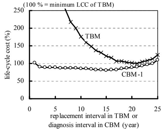
Figure 3: Relation between replacement or diagnosis interval and LCC in TBM and CBM-1
