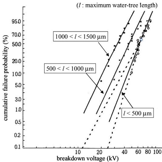
Figure 2: Weibull distribution plot of breakdown voltage for cables with different maximum water-tree length.
