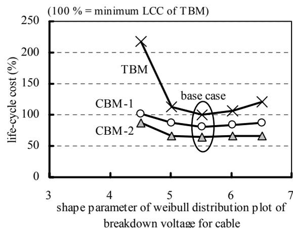
Figure 7: Increase of LCC by wrong assumption of shape parameter of weibull distribution plot of breakdown voltage.
