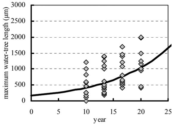
Figure 1 Relation between operation period and maximum water-tree length of CV cable.
