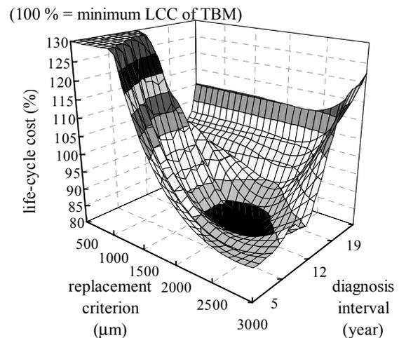
Figure 4: Relation between diagnostic condition and LCC in CBM-1.
