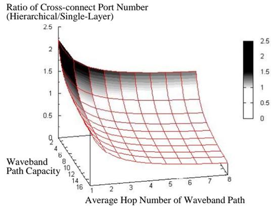
**Figure 1 Ratio of required optical ports between hierarchical and single-layer networks**
