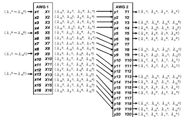
Figure 3 An example of WB MUX/DEMUX with continuous waveband arrangement
