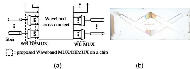
Figure 4 (a) Structure of an all-optical packet router, and (b) fabricated WB MUX/DEMUX chip using PLC technology
