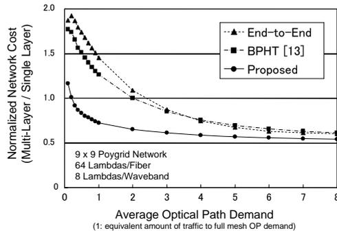
Figure 2 Comparison among proposed and conventional algorithms (end-to-end and BPHT)
