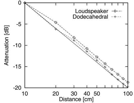
Fig. 4. Distance characteristics (Solid line represents ideal sound attenuation).
