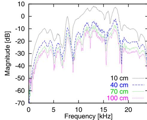
Fig. 5. Magnitude response of the impulse response at four distances (10, 40, 70 and 100 cm).
