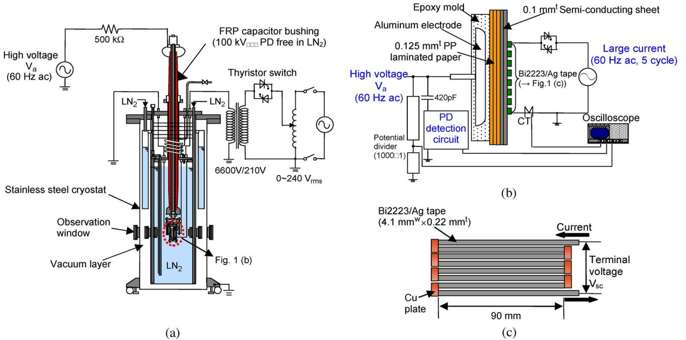
Fig. 1. Experimental setup. (a) Experimental circuit. (b) Test electrode system. (c) Bi2223/Ag tape arrangement.
