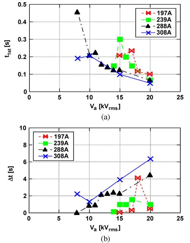
Fig. 3. PD inception time  $t_{1st}$  and PD generation duration  $\Delta t$  as a function of  $V_a$  for different  $I_{1st}$ . (a) PD inception time  $t_{1st}$ . (b) PD generation duration  $\Delta t$ .
