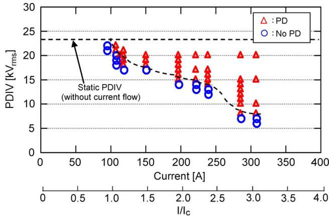
Fig. 4. Criterion of quench-induced PD generation under thermal/electrical combined stress.
