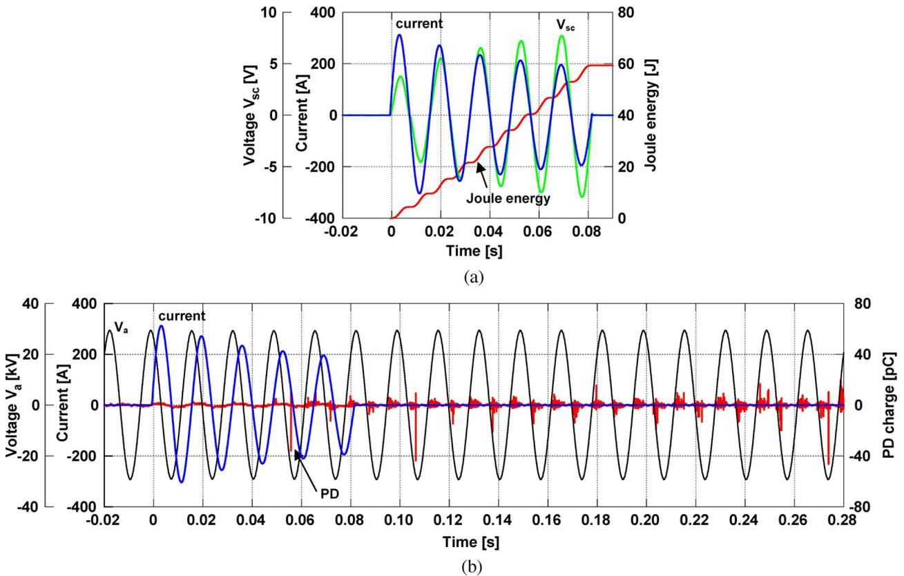
Fig. 2. Quench-induced PD phenomena. (a) Current, voltage and thermal energy waveforms at  $I_{1st} = 308 A_{peak}$ . (b) Quench-induced PD signal at  $V_a = 20 kV_{rms}$  and  $I_{1st} = 308 A_{peak}$ .
