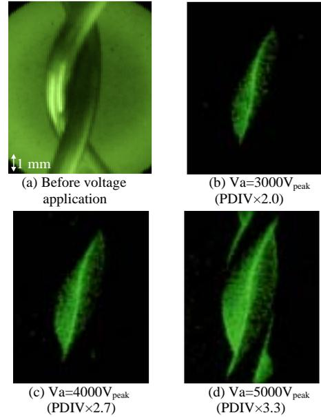
**Figure 5:** PD propagation images for 1 twisted sample (single shot)
