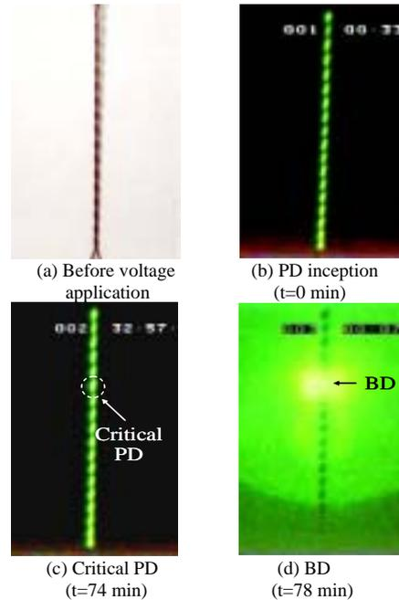
Figure 1: PD and BD light emission images for twisted pair sample.
