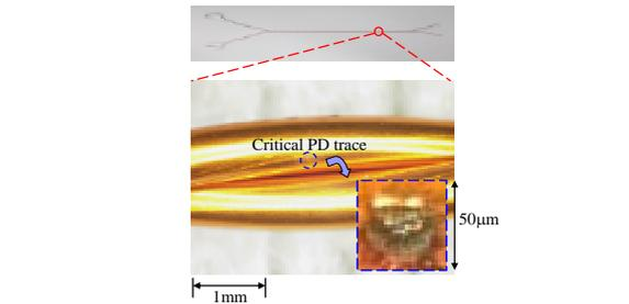
(a) Zoomed view of twisted pair with optical microscope ( $\times 100$ ).
