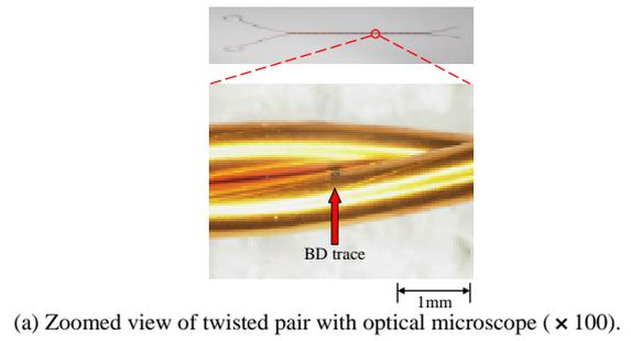
(a) Zoomed view of twisted pair with optical microscope ( $\times 100$ ).
