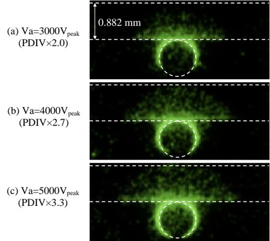
**Figure 4:** PD propagation images for point contact sample (single shot).
