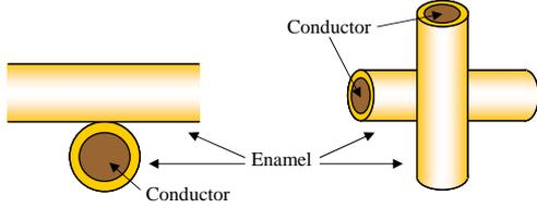
**Figure 2:** Structure of point contact sample.
