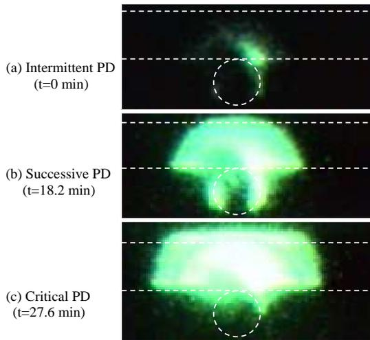
**Figure 6:** Time transition of PD light emission images for point contact sample. ( $V_a=3000V_{peak}$ ,  $f=10000pps$ , bipolar)
