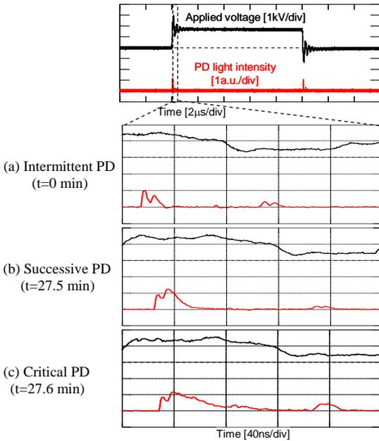
**Figure 7:** Applied voltage and PD light intensity waveforms for point contact sample.
