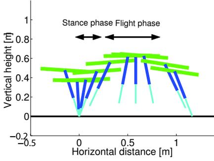
Fig. 2. Locomotion phases during one cycle
