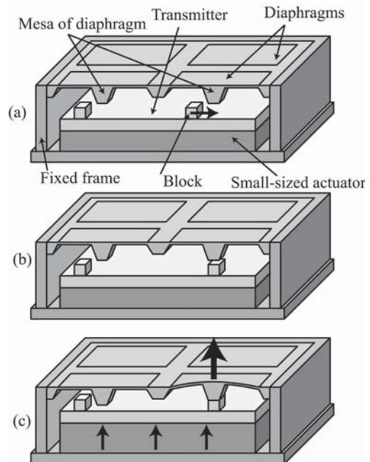
Fig. 1. Schematic view of proposed mechanical transmission system
