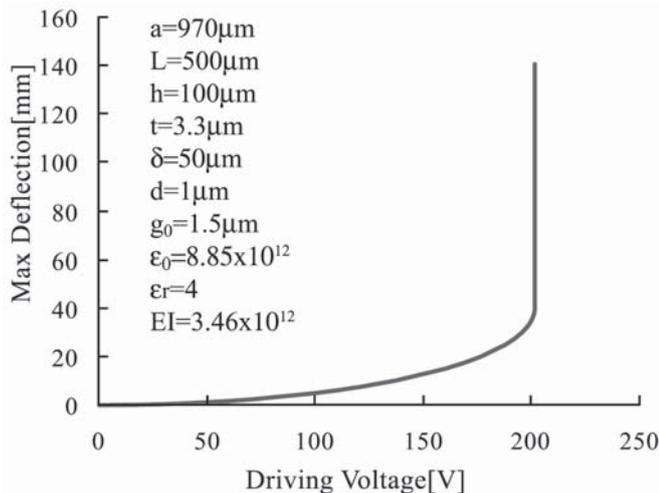
Fig. 7. Designed tulip shaped actuator deflection vs. driving voltage
