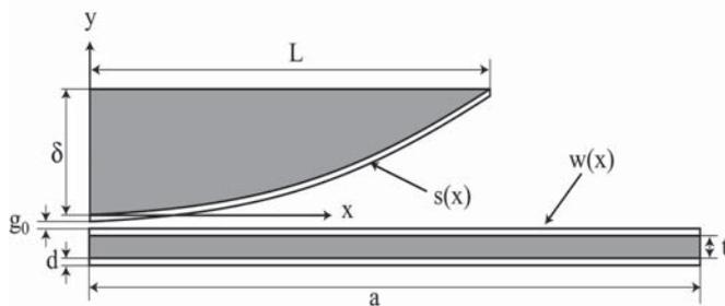
Fig. 6. Basic design of cantilever beam and curved electrode
