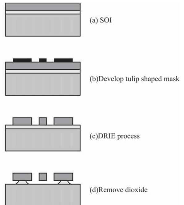
Fig. 4. Fabrication process of tulip-shaped electrostatic clutch device
