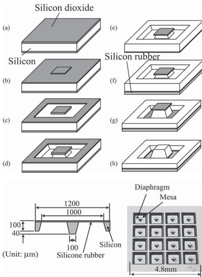
Fig. 2. Fabrication process and Fabricated arrayed end effector element
