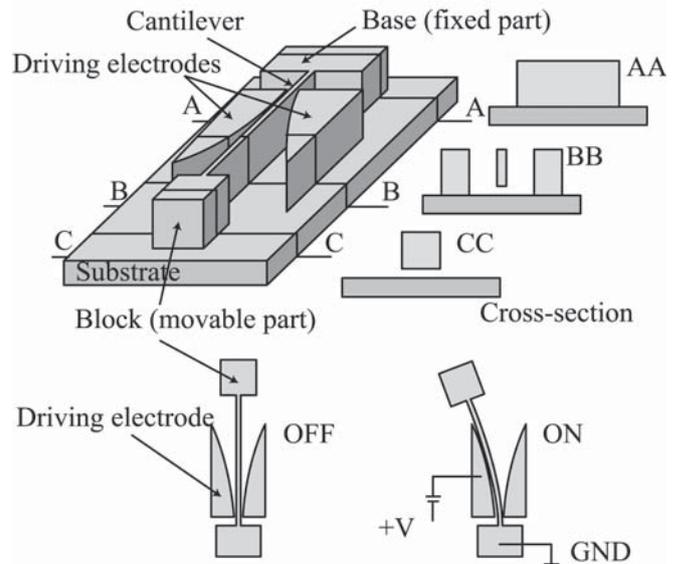
Fig. 3. Tulip-shaped electrostatic clutch device
