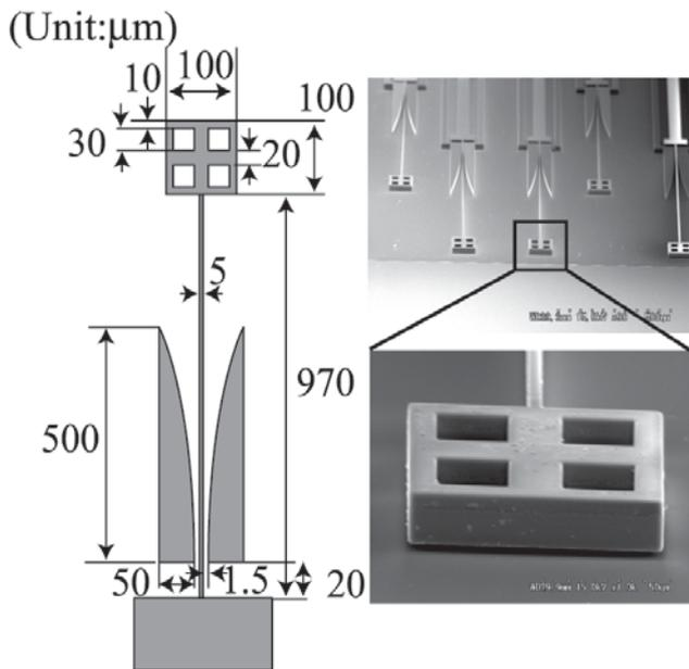
Fig. 5. Fabricated tulip-shaped electrostatic clutch device
