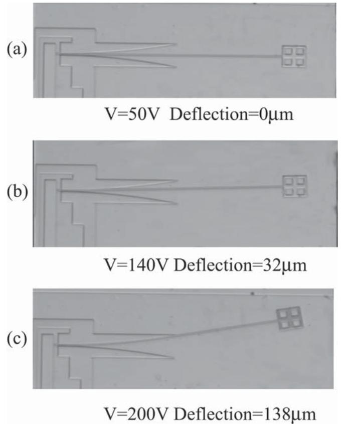
Fig. 8. Photograph of designed tulip-shaped actuator applied driving voltages of 50 V, 140 V, and 200 V
