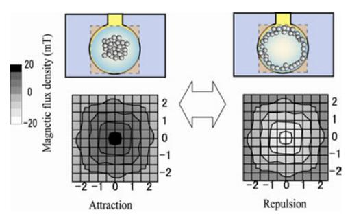
Fig. 2 Magnetic-field distribution produced by using three-layered flat coil
