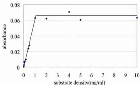
Fig. 5 Relationship between absorbance of enzymatic reacted pNPP and concentration of pNPP
