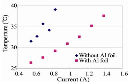
Fig. 4 Relationship between temperature inside droplet and applied current
