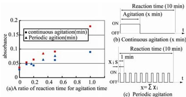
Fig. 8 Reaction dependency on agitation time
