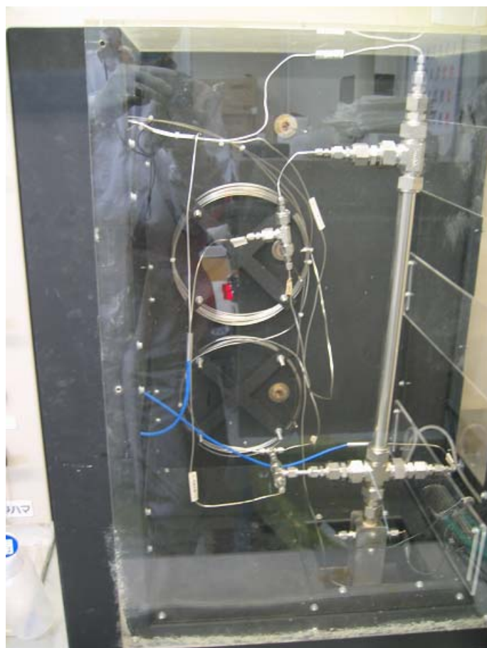
Fig. 4.4 Overview of the experimental system to strip of U(VI) in supercritical phase to aqueous phase.
