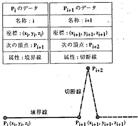
Fig. 5 Relation of paper's data and shape.
