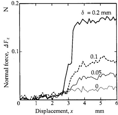
Fig. 14. Step-height detection (Going up the step).
