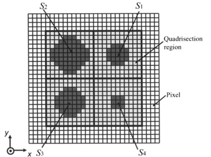
Fig. 5. Schematic view for explaining definition of quadrisection region and estimation of four contact areas.
