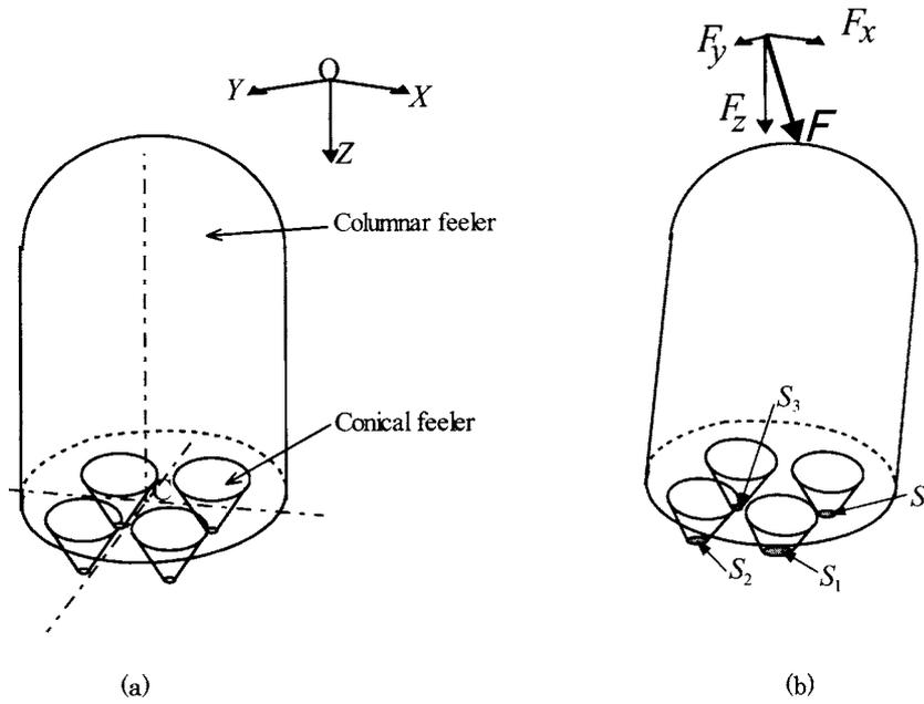
Fig. 2. 3-D view of a columnar feeler and conical feelers. (a) Initial, no force applied. (b) After force has been applied.
