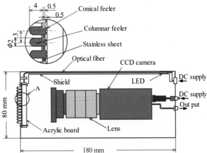
Fig. 1. Schematic of the optical three-axis tactile sensor.
