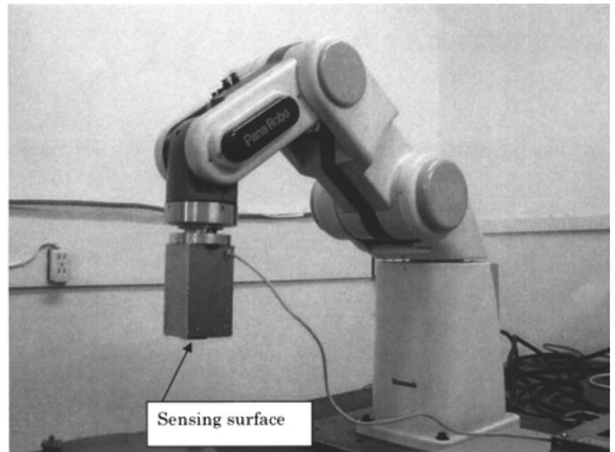
Fig. 11. Robot equipped with the three-axis tactile sensor.
