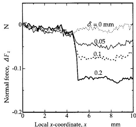
Fig. 15. Step-height detection (Going down the step).
