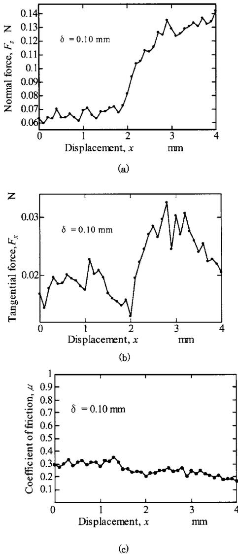
Fig. 13. Estimation of the best parameter for step-height presentation. (a) Normal force,  $F_z$ . (b) Tangential force,  $F_x$ . (c) Coefficient of friction,  $\mu$ .
