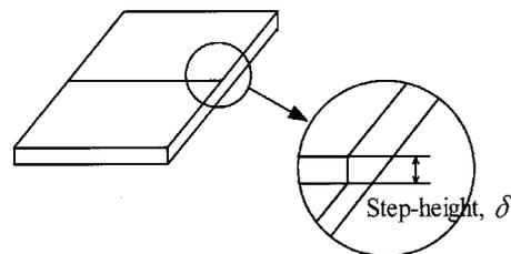
Fig. 12. Specimen having step-height.
