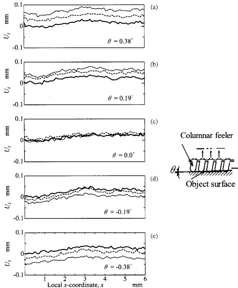
Fig. 16. Outputs of three sequential feelers under inclination detection.
