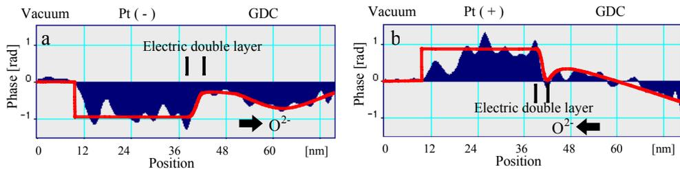
Fig.4. Phase differences between that of -1.0V and 0 (a), and that between +1.0V and 0 (b) show electric double layers and localization of oxygen anions. Solid red lines correspond to electrostatic potential.
