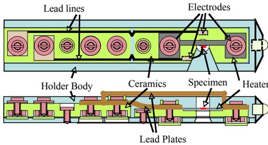
Fig.1. New specimen holder with 4 electrodes.
