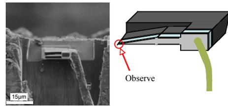
Fig.2. Specimen mounted on the side edge of the heater.
