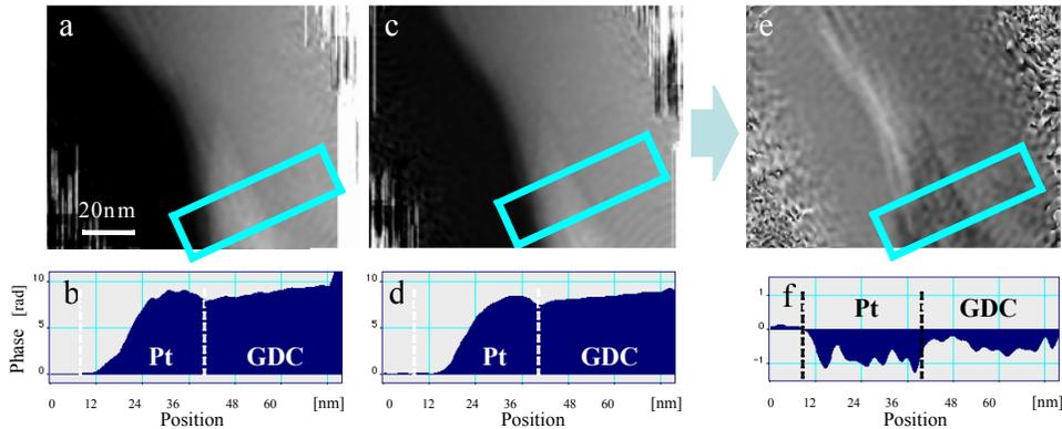
Fig.3. Reconstructed phase images and their line profiles, (a) and (b):without an external field, (c) and (d): with applying -1.0V to the Pt electrode, (e) and (f):subtracted (a) from (b). Frames are areas averaged for profiling.
