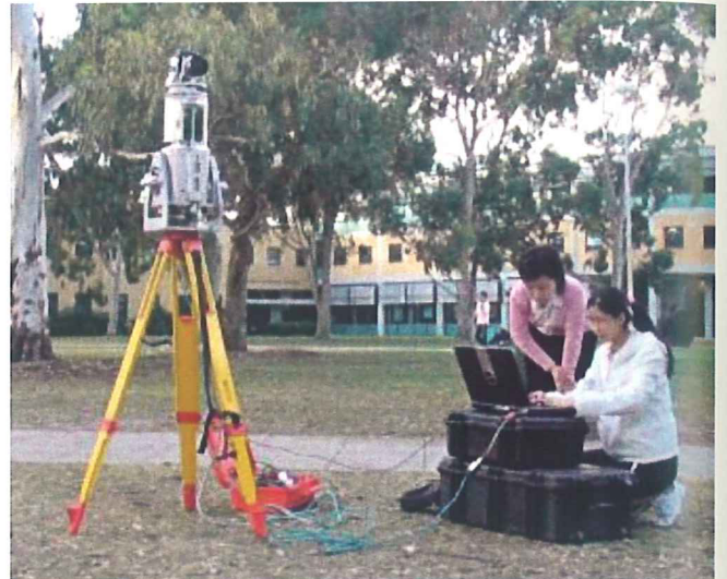
Figure 2 Large scale laser scanner - Riegl LMS420i - note the color Nikon camera on top of the laser to capture the color information augmenting the depth information from the laser.
