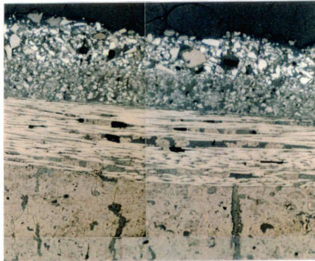
Fig. 2-3-6 Photograph of cross section of the No. 3 specimen after oxidation test at 1773K in air for 10 hrs
