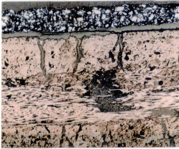
Fig. 2-3-5 Photograph of cross section of the No. 3 specimen before oxidation test
