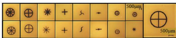
Figure 8: Photos of magnetic micro-rotors used in the micro-stirrer on a chip.
