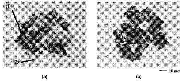
Fig. 2 Photograph of mixture of fly ash and PE : Temperature, 523K ; Mixing time, 20min (a) Mixing ratio ; PE 1.5g/fly ash 10g (b) Mixing ratio ; PE 2.5g/fly ash 10g
