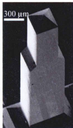
Fig.1 SEM image of SiC tip that was cut out from a SiC single crystal.
