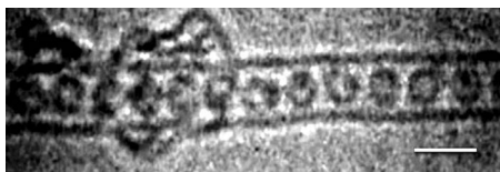
FIG. 1. A HRTEM image of (\text{Gd}@C_{82})@SWNT . The scale bar is approximately 2 nm.
