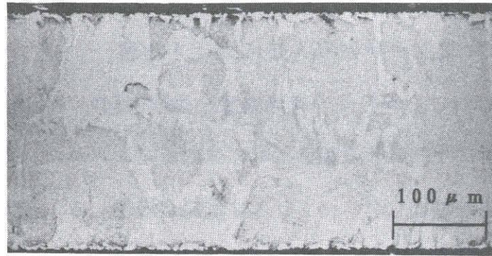
(A) Treating time:1.8ks, Plasma current:0.02A Carbon content:0.35mass%
