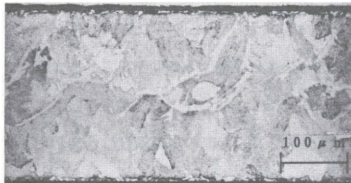
(B) Treating time:3.6ks, Plasma current:0.03A Carbon content:0.77mass%
