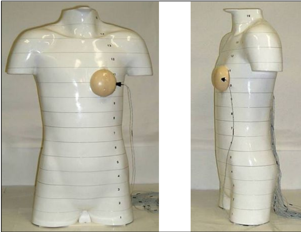
Figure 2-1 Dosimeter implanted anthropomorphic phantom.
