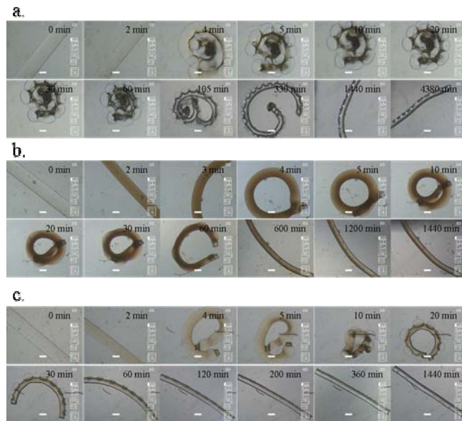
Figure 3.13. Optical micrographs of morphological changes during shrinking of sub-micrometer sized cylindrical a.) TN(2) b.) R w N(2) and c.) R ws N(2) hydrogels after a temperature jump from 20 °C to 40 °C
