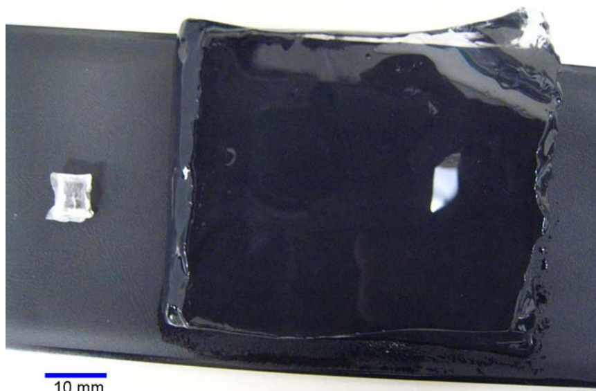
Figure 4.15. Volume change of R_{ws}N-S0.8 gel in water. Left: the dried gel (129 mg) and right: the water-swollen gel (80g) The R_{ws}N-S0.8 gel absorbs water up to ca. 62,000 wt% to its dried state.
